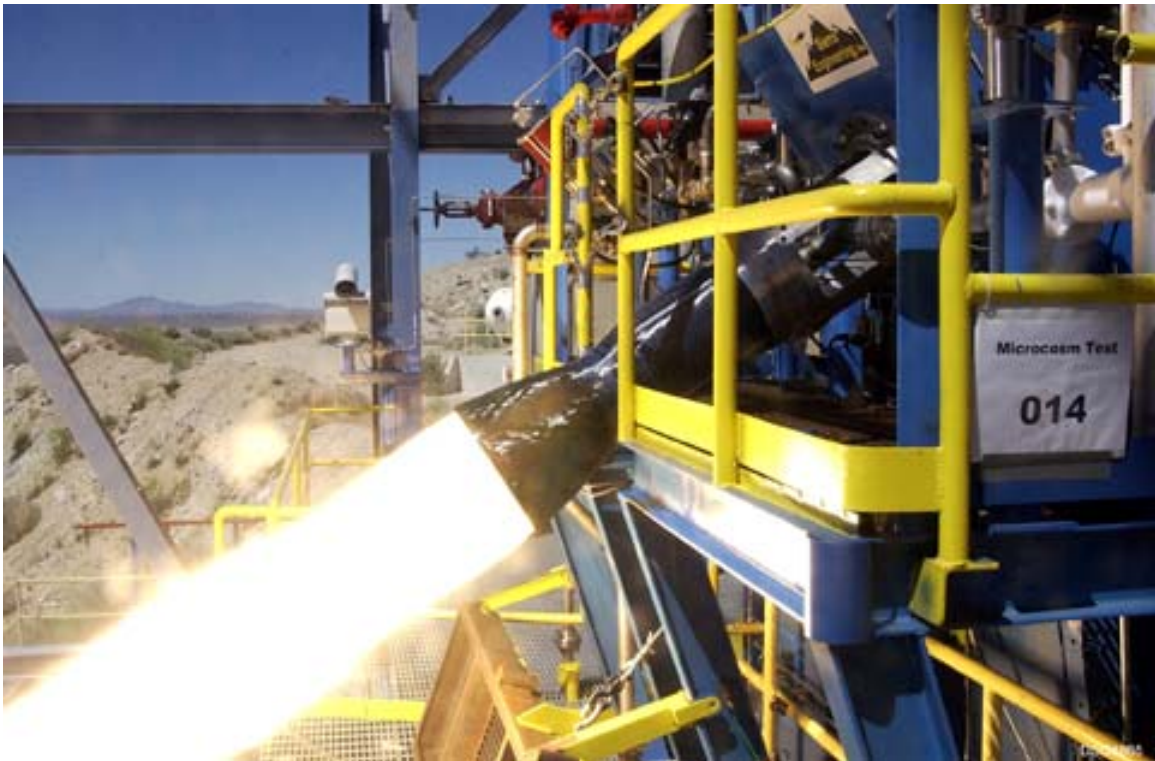
Microcosm 20,000 lbf rocket engine undergoing testing at the Air Force Research Laboratory facilities at Edwards Air Force Base, CA, May 21, 2005.
