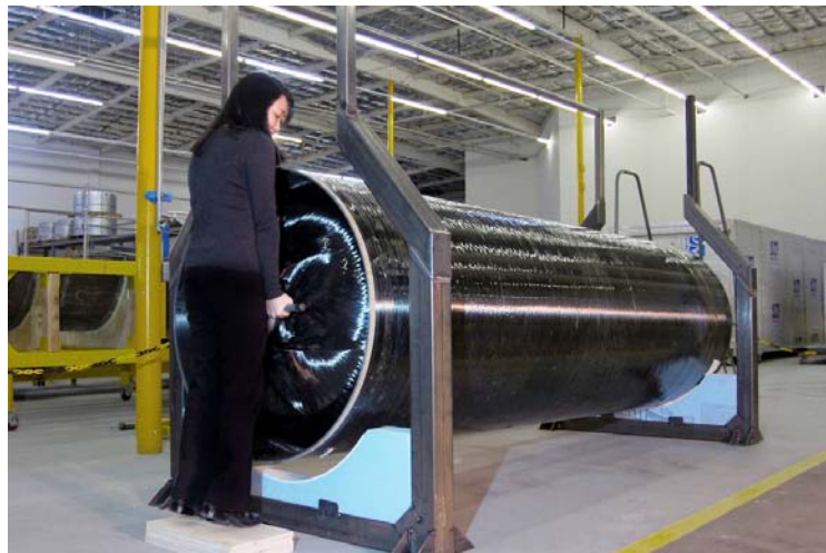
The composite tank is both strong and light weight. By picking up one end, Lynn, who works in the Microcosm business office, is lifting half the weight of the tank (without the pick-up or engineering crew on top). Notice that even though we gave her a 2x8 to stand on, she's still on tip toes lifting the tank.
