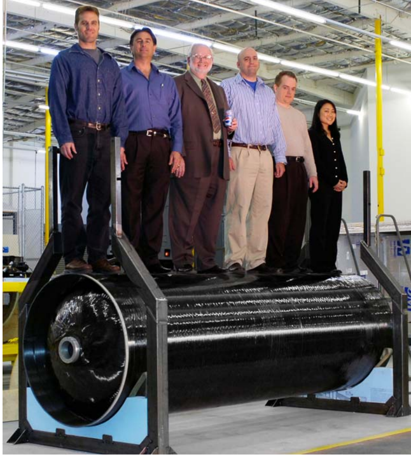
The Microcosm engineering crew is on top of their work. This is the prototype LOX tank for the Sprite Small Launch Vehicle, a member of the Scorpious® family of responsive, low-cost launchers. From left, Dana, Keeler, Blake Bartosh, Jim Wertz, Aaron Leichner, John Collins, and Lynn Shimohara.
