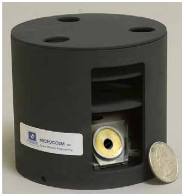
Figure 2. MicroMak Model with Internal View Showing Optical Head Position Inside along with Light Baffling Structure (internal plates above optical head). (Note: The rectangular “window” is only to show internal structure and is not part of the design for operational sensor.)
