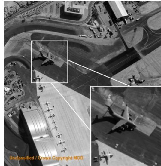
Fig. 2. Image quality expected from the Goodrich SYERS-derived payload flying at an altitude of 200 km.
