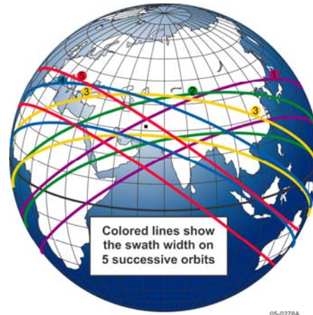
Fig. 1. A Repeat Coverage Orbit Provides a Short Span of Coverage of a Defined Region on 5 or More Successive Orbits. This type of responsive orbit provides a high level of utility for monitoring or tracking ground activity at a specific time in a specific region and would be disruptive to enemy operations if an attempt were made to avoid surveillance. [Wertz, 2005]
