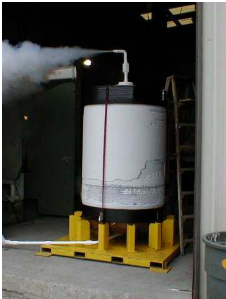
Figure 3: All-Composite LOX Tank (left) in Cryogenic Testing and Flight-Proven Fuel Tank (right).
