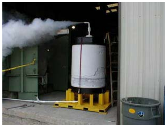
Fig. 6. All-Composite LOX Tank (top) in Cryogenic Testing and Flight-Proven Fuel Tank.
